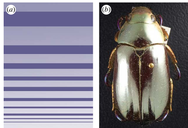
Figure 5. Broadband multilayer reflectors. (a) Schematic of chirped reflector and (b) broadband reflectance in Chrysina chrysagryrea (Scarabaeidae: Rutelinae).
